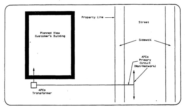
Designated Underground Area · Building Set Back From Property Line · Primary Underground to Transformer Located Outside of Building · Secondary Underground Service · Secondary Metering
