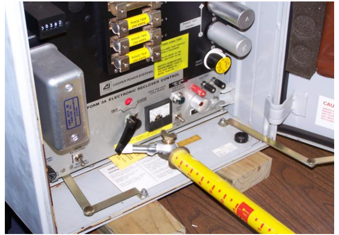
Push button hot stick attachment placed at an angle to give more leverage. Can be used on smaller type 101 control switches.
