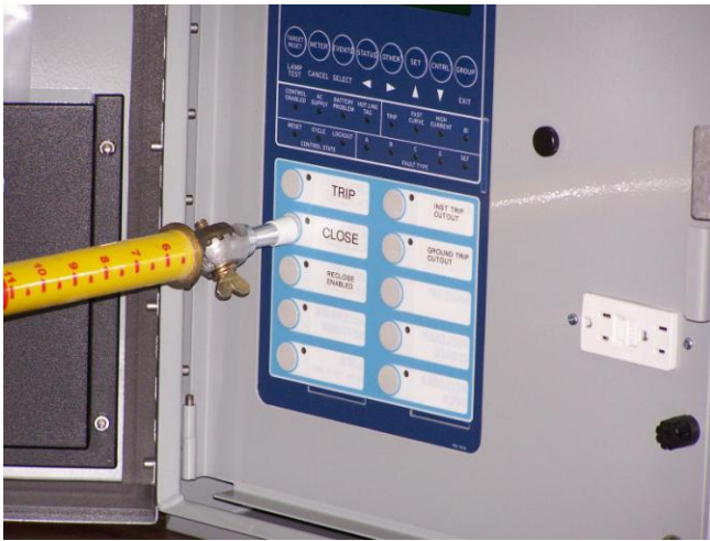
Push button hot stick attachment to be used on push button type control switches that do not have time delay trip and closing.
