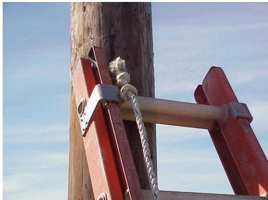
**Step 1:** Tie one end of a rope to the top rung of the top section of the ladder.
